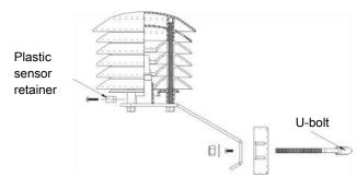
Loosen the plastic sensor retainer on the radiation shield by unscrewing two retainer screws.
